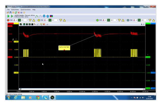
My first thought was that one of the control units was causing interference to the signal which of course was affecting the complete network so next was the painstaking job of disconnecting each control unit in turn with the scope still connected to see if the signal improved with the units plugged out.
