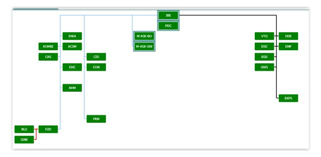
JBE (Junction box Electronics) FRM(Football Module) CAS (Car Access System) CON (I drive controller) CID (Central Information Display) EHC (Electronic Height Control) KOMBI (Instruments Cluster) PDC (Park Distance Control) FZD (Roof Control Panel) MASK (Radio Head Unit) IHKA (Air Conditioning Control Unit)
