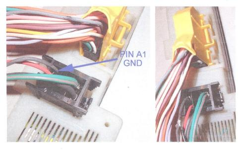
Ignition: Red wire on Record / Playback module to Pin 6 on Yellow 26 way connector (usually a yellow wire)
