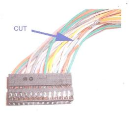
Finally, if you wish to disable the red security LED on the dashboard, you need to cut the wire to pin 24 of the connector above. It's usually white, but again see the note below.
