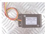
If you can disarm the original immobiliser once, either by entering the over-ride pin, or by substituting components (e.g. a working infra red receiver), it's possible to program the Record and Playback Module without any other specialist tools.
