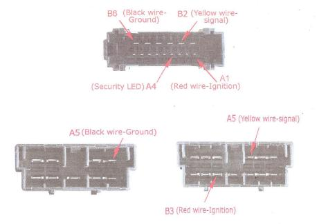
**Step 2 - Recording:** Once the module is wired to the vehicle, turn Ignition ON and the Yellow LED on the module will come ON. This signifies that the module is ready to start recording. De-activate the immobiliser by PIN entry or other method and the module will learn, the code sent by the immobiliser. For Software version 1.1, connect the yellow wire at this point in time.
