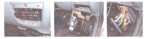
All the connections shown need to be made to connectors on the top (black) face of the unit.
