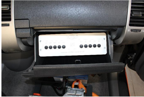
Fault simulator switches in the car trunk
