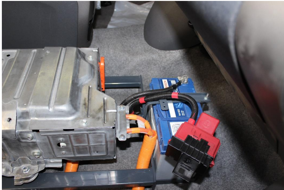
Installation location for 12 V and high voltage storage batteries
