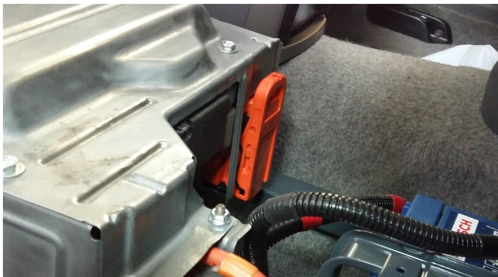
Maintenance connector (in the middle of the picture, orange)
