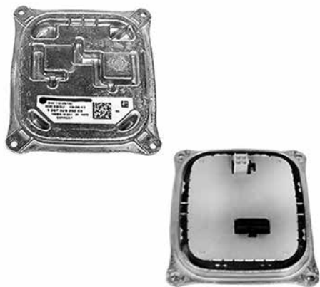
DRL LED control unit
