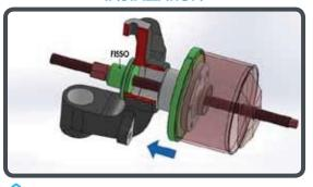
Pulling rings system - when closed - allows to push around the external diameter of the bearing, in the undercut granting the perfect operation of the product, avoiding the break of the hub
