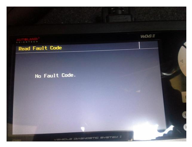
So now it proved that the wiring back to the control unit was fine and the module was also fine so it had to be the safety battery terminal that was at fault
