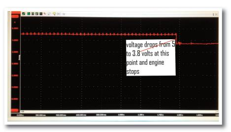
Voltage supply to some sensors dropped from 5v to 3.8v whenever the engine stopped
