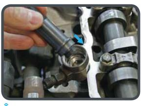
Fixing to the injector inner part with M14x1 adaptor.
