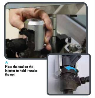
if necessary, unscrew the FIXING NUT slightly to have the space necessary to place the tool.
