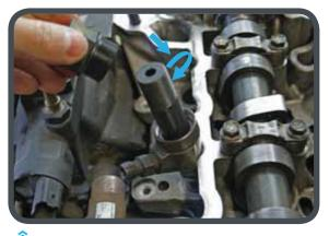
Fixing to the injector's external nut M25x1.
