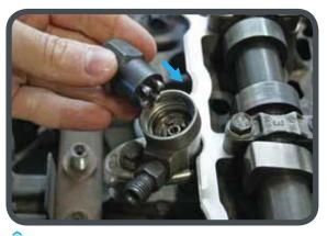
Dismantling the inner part of the injector.
