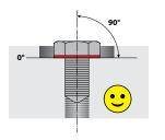
Defective seal seat, no longer flat! Thread alignment not exactly at 90° respect to the sealing surface.
