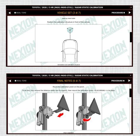
SCE 300 is intuitive, the PROADAS software guides the operator through the various system alignment procedures avoiding positioning errors; it is **compatible with official OEM and Multibrand diagnostics** (in this case the specific ADAS sensor must be managed within the diagnostic device).
