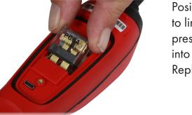
Position the new Circuit Breaker into the housing, take care to line up the breaker spades with the breaker terminals, and press down gently until the Circuit Breaker is fully engaged into the breaker terminals.
