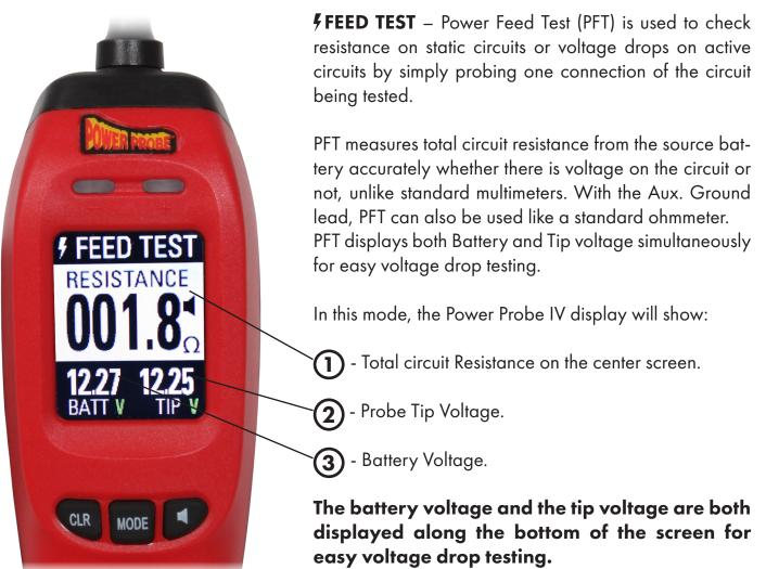
The circuit resistance will be calculated even with voltage applied to the circuit. To accurately test the power and ground feed resistance, the component must be removed from the circuit first. Simply unplug any component, relay, or module on the circuit, contact the probe tip to the circuit and view the circuit resistance.
