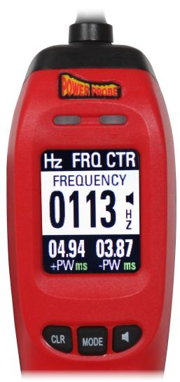
**Hz FRQ CTR** – Frequency Counter mode is used for measuring the frequency of an alternating voltage signal.
