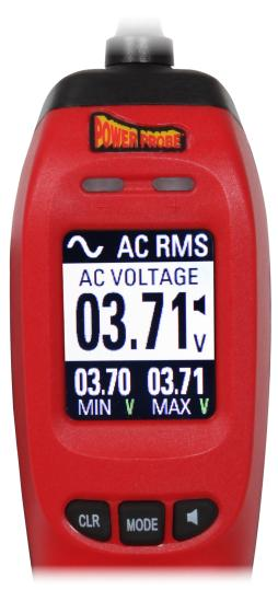
▲ AC RMS mode is for measuring AC (alternating current) voltages and can be used on any AC voltage or pulsed waveform signal where an RMS averaged voltage measurement is required.
