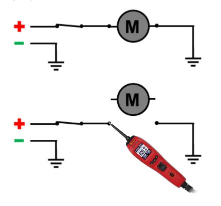
Remove component from circuit before performing Power Feed Test
