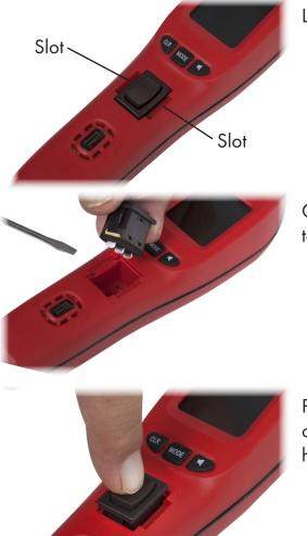
Locate the two slots on either side of the Rocker Switch.
