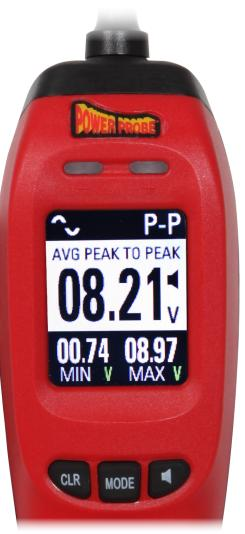
**^ P**-**P** mode can be used on any AC voltage signal where a Peak to Peak (P-P) voltage measurement is required.
