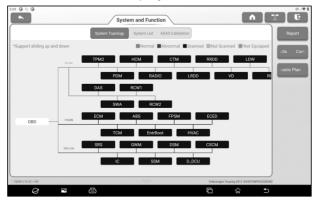
The user can manually select the vehicle electronic control system to perform the test function operation. Click a single electronic control system (such as "ECM") in the test option selection interface, and then tap **Enter** to go to the test function selection page.
