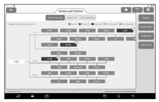
The system with fault codes will be displayed with red background, and the specific number of fault codes will be displayed. Click on a single system to view specific fault information. No fault system will be displayed with green background.
