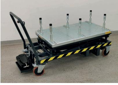
Used for platforms with M8 and M10 threaded holes
