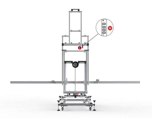
1. Turn on the altitude range-finder ① and adjust the device height to make the value of altitude rangefinder ① is H, H=\_\_\_\_\_.
