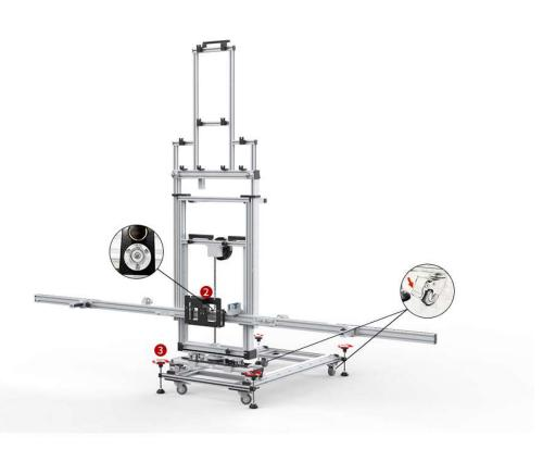
5. Observe the spirit level ②, rotate the base adjustment knob ③, and lock the moving wheels after the device is leveled.
