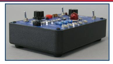
The Electrical/PWM/Fault Trainer is designed to introduce the concepts of Electrical Fundamentals, Pulse Width Modulation (PWM) Actuator Control, and Fault Diagnosis. The trainer is compact, self-contained, and provides a PWM output to view the signal on an
